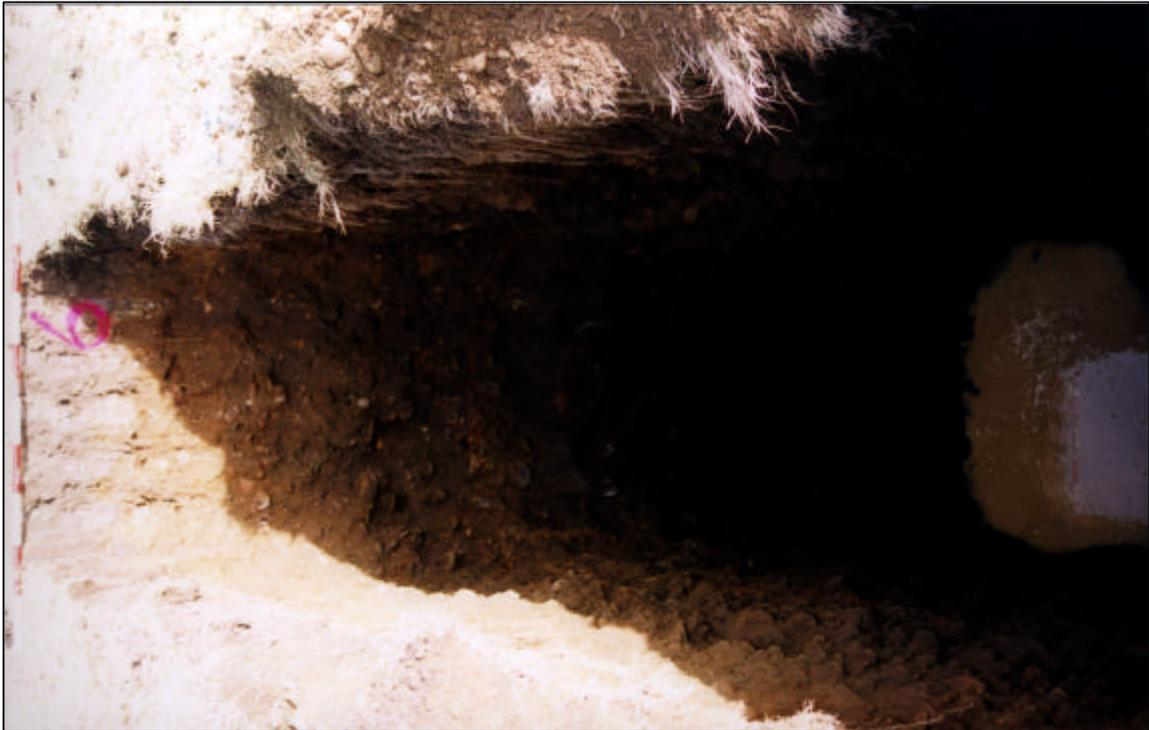
Test Pit 6 showing yellow brown silty gravel. Water table is at about 4 m
