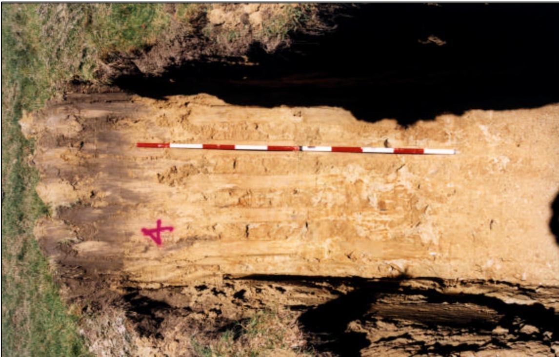
Test Pit 4 showing yellow brown loess colluvium containing rare gravel clasts overlying gravel.
