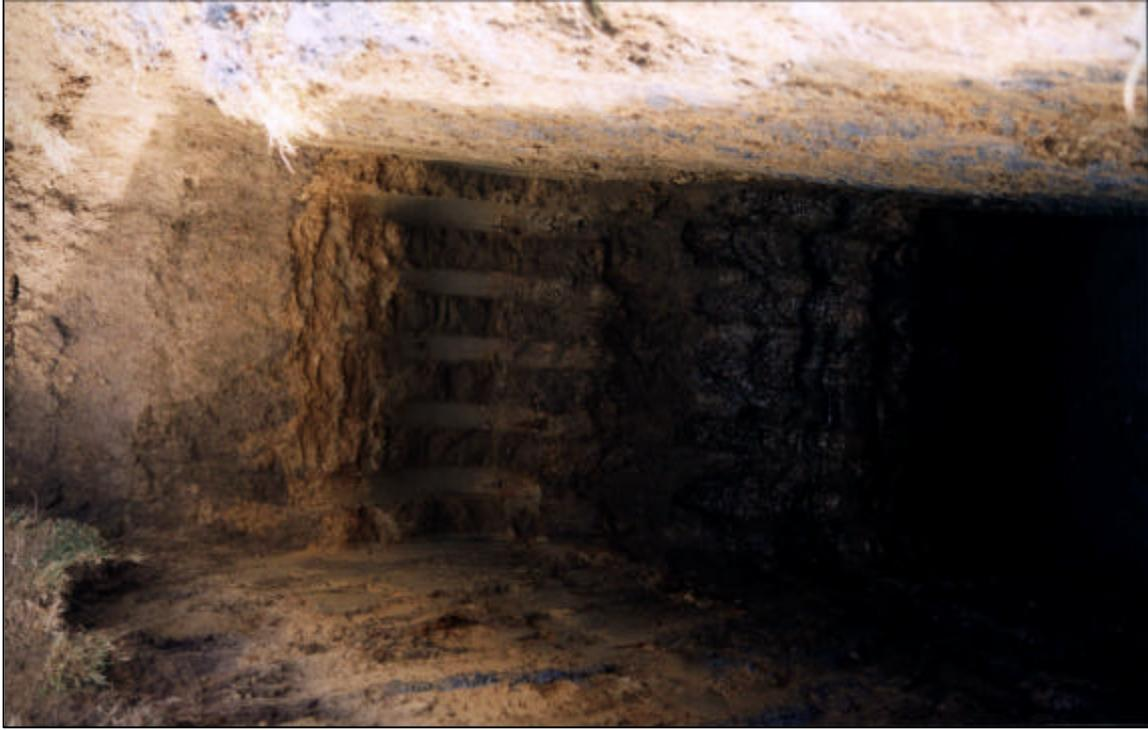
Test Pit 7 showing interbedded sand, silt and pebbly gravel. Water table is at about 4 m depth.
