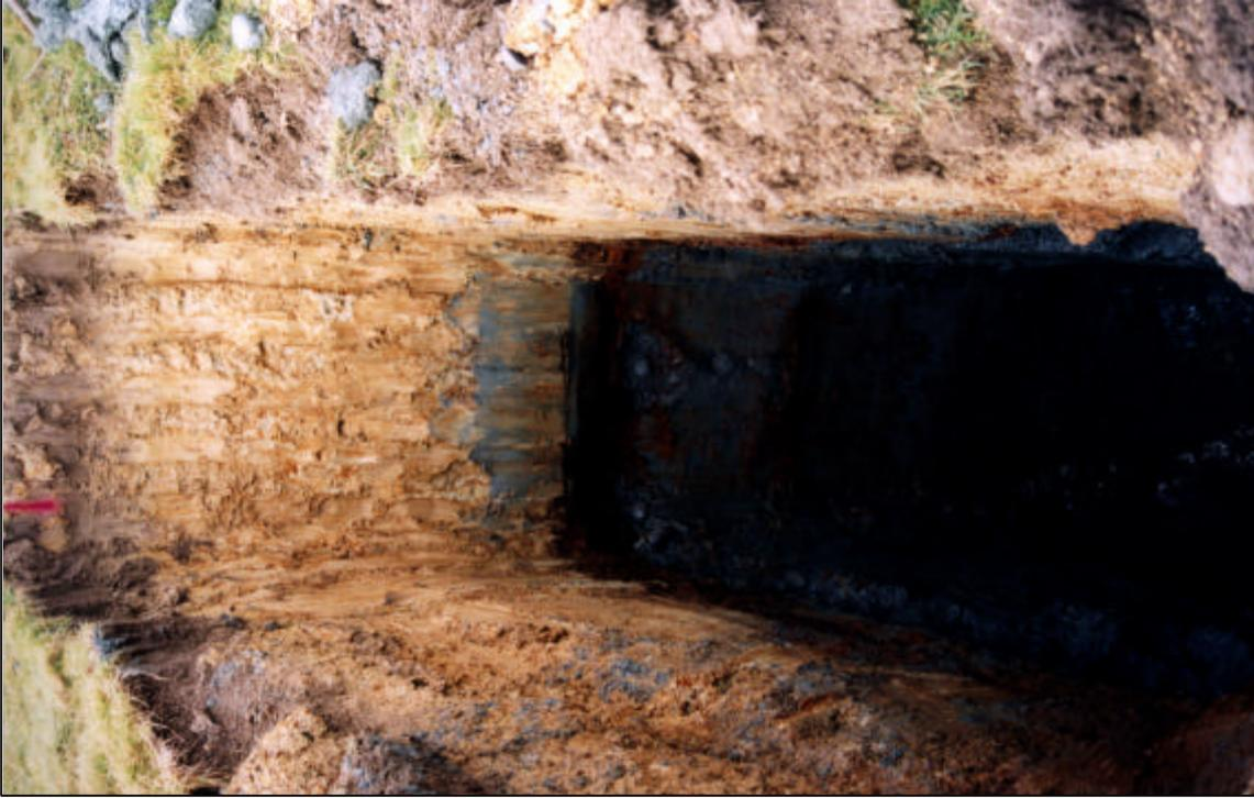
Test Pit 1 showing brown gravelly silt overlying saturated grey silts and gravels
