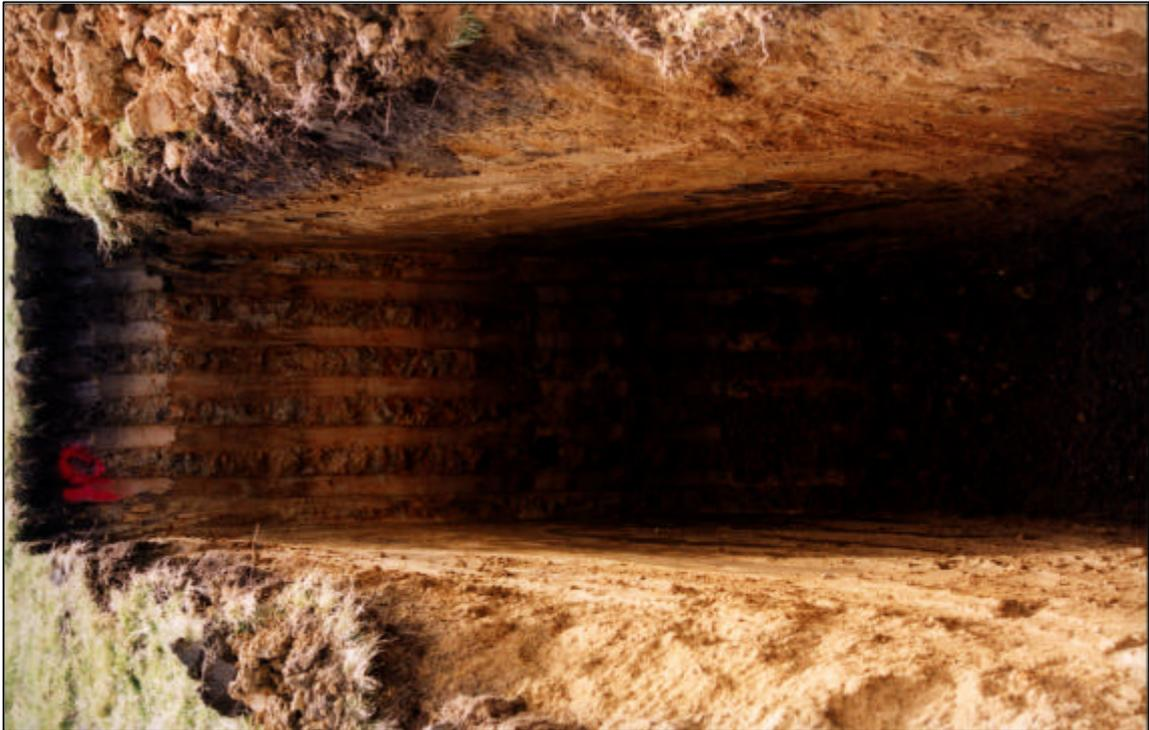
Test Pit 10 showing yellow brown loess overlying weathered gravel at about 3 m depth.
