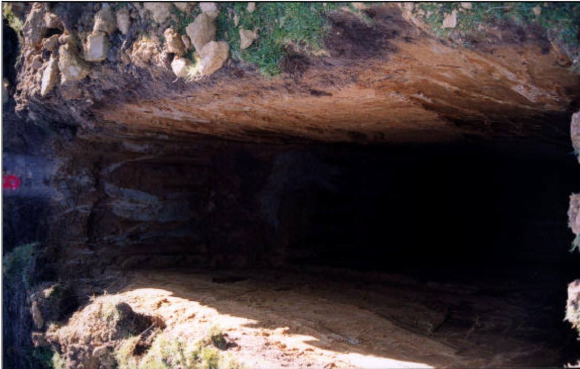
Test Pit 8 showing yellow brown loess to the full excavation depth of about 6 m.
