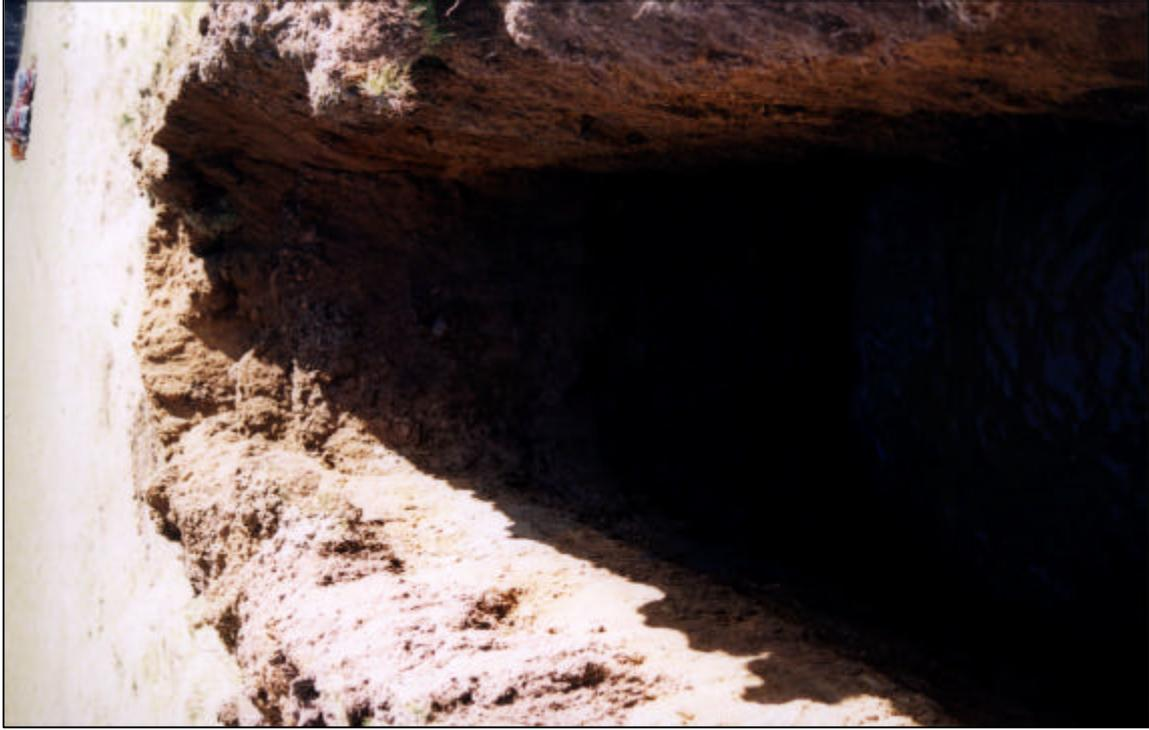
Test Pit 5 showing interbedded sand, silt and pebbly gravel. Water table is at about 2 m depth.
