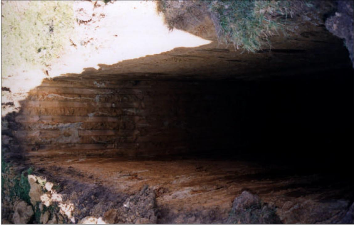
Test Pit 9 showing yellow brown loess to the full excavation depth of about 5.5 m.
