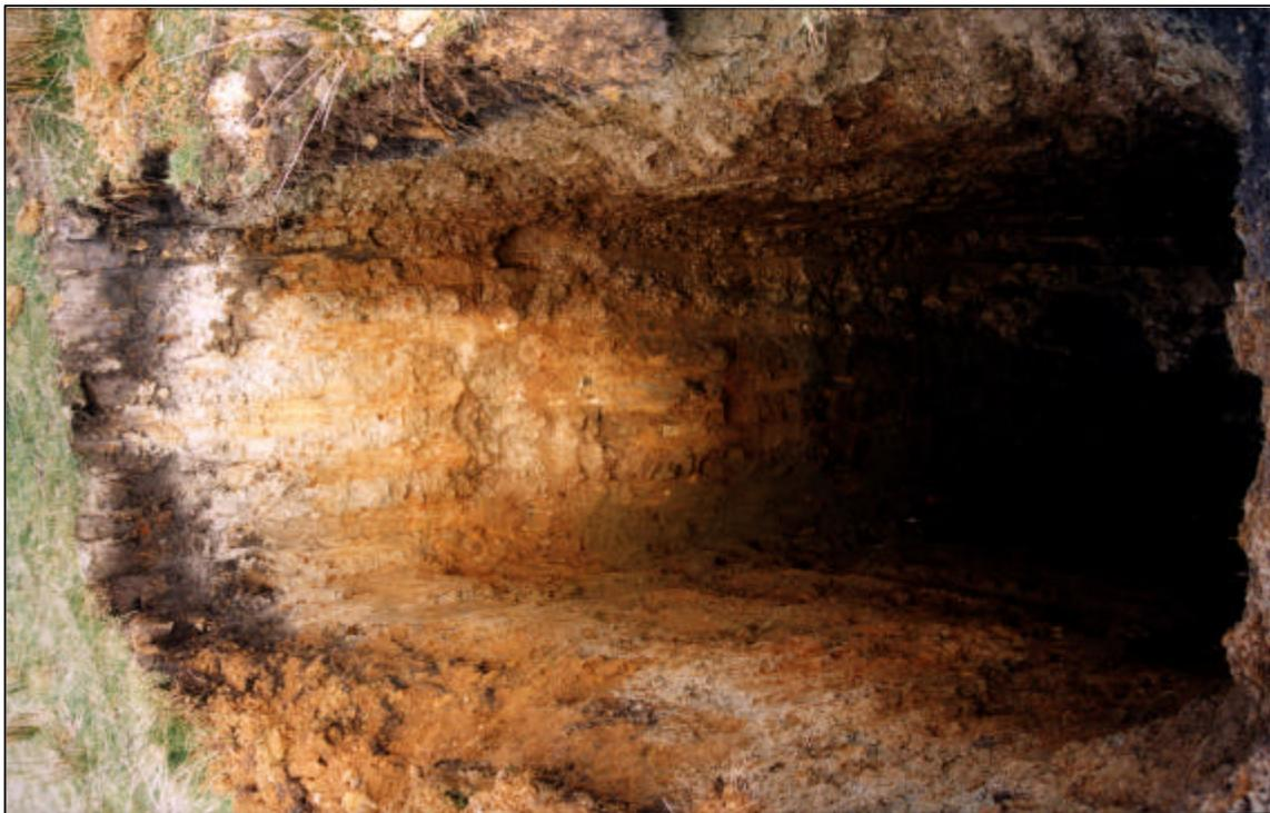
Test Pit 11 showing yellow brown silty gravel colluvium overlying grey sandstone at about 3.0 m.
