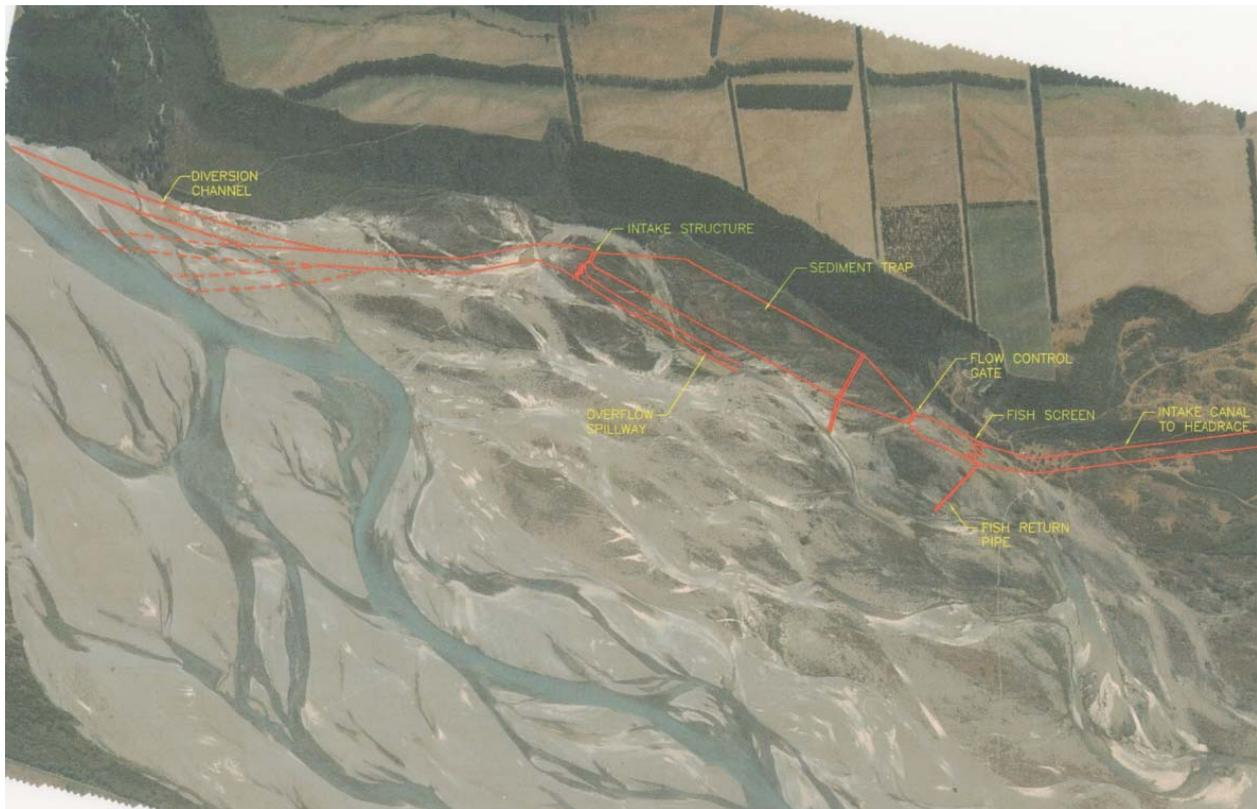
FIGURE 3-4: Rakaia River Intake (Scheme features shown at approximate locations)
