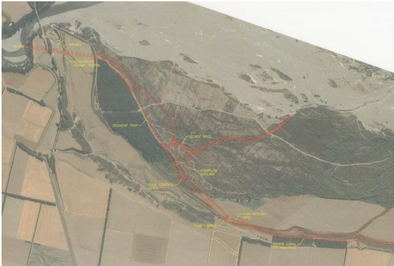
FIGURE 3-5: Waimakariri River intake – lower site (Scheme features shown at approximate locations)
