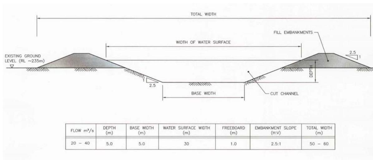
FIGURE 3-11: Cross section of the headrace
