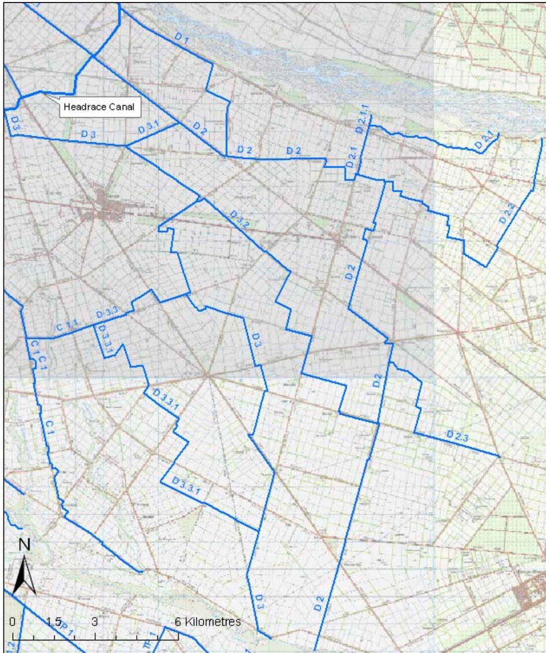
FIGURE 3-17: Darfield water distribution race network
