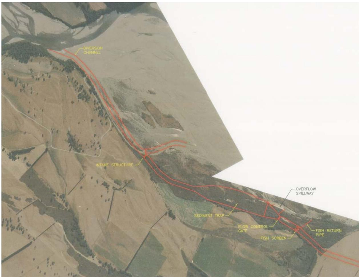
FIGURE 3-6: Waimakariri River intake – upper site (Scheme features shown at approximate locations)
