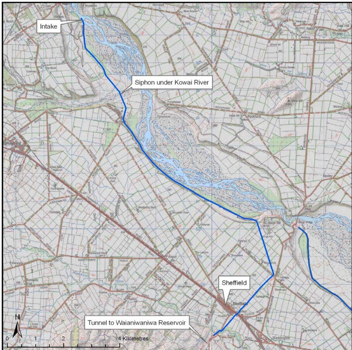
FIGURE 3-7: Alignment of the Inlet Canal to Waianiwi Valley
