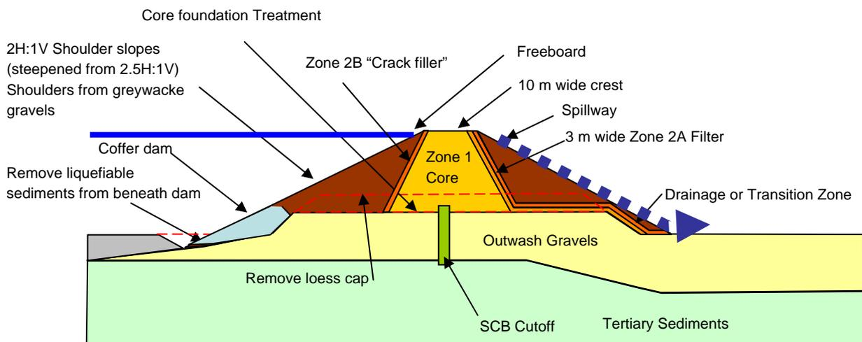
FIGURE 3-9: Typical cross section of the embankment dam
